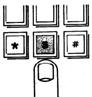
To arm with zone(s) shunted, first check the green STATUS lamp to make sure that no perimeter zone is in "trouble". Then press the SHUNT button, labeled "S", and enter your code. The yellow SHUNT light and the red ARMED/MEMORY light will come on. The green light will go out when you disarm the Control Center.
