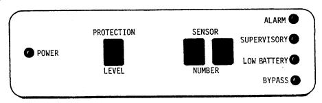
ALARM - The identifying number of the sensor in alarm is displayed in the Sensor Number window while the ALARM light is on.
